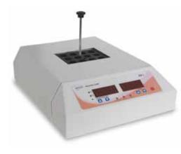
COD Heater Block, 120V and 230V, 12-tube capacity
