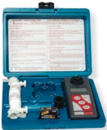
Pocket Photometer with Case and PPD-2 DPD Dispensers
